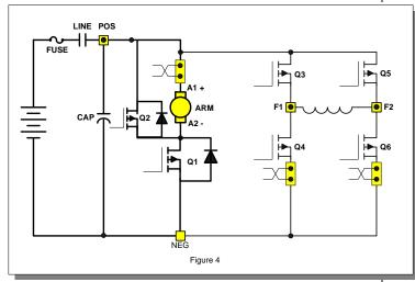
By energizing the transistors in pairs, current can be made to flow in either direction in the field. The armature control circuit typically operates at 12KHZ to 15KHZ, a frequency range normally above human hearing. This high frequency coupled with the elimination of directional contactors, provides very quiet vehicle operation. The field control circuits typically operate at 2 KHZ.
